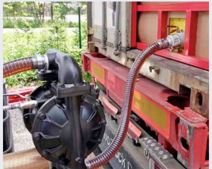
High fluid viscosity reduces pump delivery.
